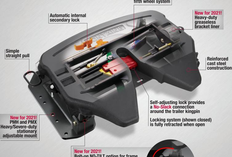
**Bolt-on NO-TILT option for frame** dump applications—Simply flip the four levers on the mount to prevent the fifth wheel from rocking
